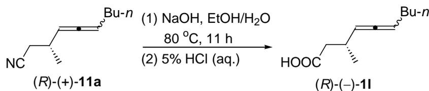
Following the procedure for the preparation of **6a**, the reaction of (*R*)-(+)-**11a** (0.3456 g, 2.1 mmol), ethanol (8 mL), and NaOH solution (2.0014 g in 2.5 mL of H<sub>2</sub>O, 50 mmol) afforded (*R*)-(–)-**11** (0.2988 g, 77%, *dr* = 1.2/1): liquid, the <sup>1</sup>H NMR data are the same as those for (*S*)-(+)-**11**. [ $\alpha$ ]<sub>D</sub><sup>20</sup> = -12.5 (*c* = 1.24, CHCl<sub>3</sub>).
