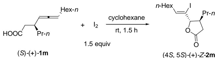
The reaction of (*S*)-(+)-**1m** (34.9 mg, 0.15 mmol) in cyclohexane (2 mL) with I<sub>2</sub> (57.2 mg, 0.225 mmol) afforded (4*S*, 5*S*)-(+)-*Z*-**2m** (38.2 mg, 72%, *Z*/*E* = 96/4, 99% ee, HPLC conditions: Chiralcel OJ-H column; rate, 0.5 mL/min; eluent, hexane/*i*-PrOH = 95/5; λ = 254 nm, t<sub>R</sub> 11.9 (minor), 12.9 (major)). The <sup>1</sup>H NMR data are the same as those for racemic *trans*-*Z*-**2m**. [α]<sub>D</sub><sup>20</sup> = +40.0 (*c* = 1.2, CHCl<sub>3</sub>).
