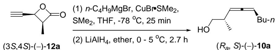
To a solution of CuBr·SMe<sub>2</sub> (6.8 mg, 0.03 mmol) and dimethylsulfide (0.2 mL) in
