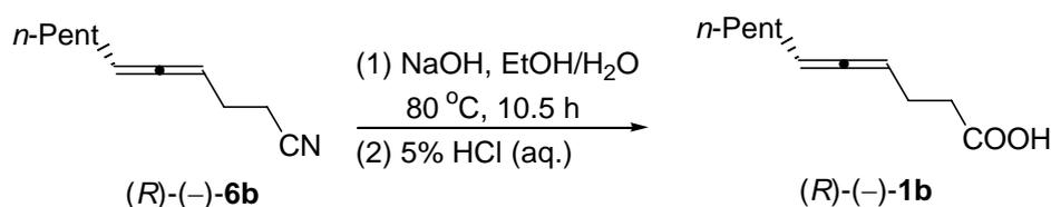
The reaction of (*R*)-(-)-**6b** (1.0121 g, 6.2 mmol), ethanol (15 mL), and NaOH solution (4.0 g in 5.3 mL of H<sub>2</sub>O, 100 mmol) afforded (*R*)-(-)-**1b** (1.1434 g, 100%): liquid, <sup>1</sup>H NMR (300 MHz, CDCl<sub>3</sub>) δ 10.61 (bs, COOH, 1H), 5.20-5.11 (m, 2H), 2.54-2.42 (m, 2H), 2.35-2.24 (m, 2H), 2.01-1.92 (m, 2H), 1.44-1.34 (m, 2H), 1.34-1.20 (m, 4H), 0.88 (t, *J* = 6.8 Hz, 3H). [ $\alpha$ ]<sub>D</sub><sup>20</sup> = -76.7 (*c* = 1.05, CHCl<sub>3</sub>).
