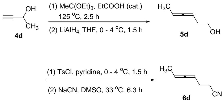
But-3-yn-2-ol (**4d**) (7.5 g, 0.11 mol) was added dropwise to the mixture of EtCOOH (1.6 mL, *d* = 0.99 g/mL, 1.58 g, 0.021 mol) and MeC(OEt)<sub>3</sub> (48.0 g, 0.30
