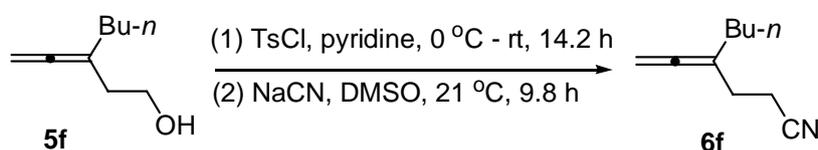
Following the procedure for the preparation of **6a**, the reaction of **5f** (2.8065 g, 0.020 mol), *p*-TsCl (11.5 g, 0.060 mol), and anhydrous pyridine (30 mL) afforded the tosylate, which was used in the next step without further purification. The reaction of tosylate prepared above and NaCN (1.1860 g, 0.024 mol) in anhydrous DMSO (25 mL) afforded **6f** (1.5671 g, the combined yield from **5f** to **6f** is 52%): liquid,  $^1\text{H}$  NMR
