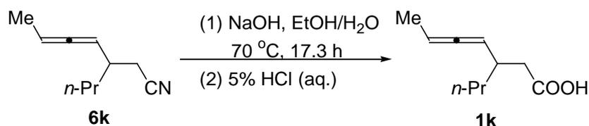
Following the procedure for the preparation of **1a**, the reaction of 3-propylhepta-4,5-dienitrile (1.0073 g, 6.8 mmol), ethanol (15 mL), and NaOH solution (4.0 g in 5.2 mL of  $\text{H}_2\text{O}$ , 100 mmol) afforded **1k** (0.6690 g, 59%,  $dr = 2.2/1$ ,
